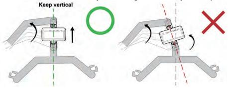
Even if Lift Scale is completely vertical when installed, if it is bent at any point in operation (ex: Patient Lift System raises patient to higher point for weight measurement), the same risk of breakage applies.
