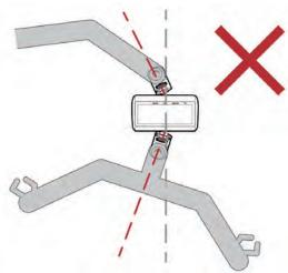
If any visual damage or bending is observed, do NOT use Lift Scale.
