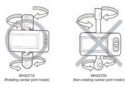
The cardan joints on MHS2710 Lift Scales (with **rotating** cardan joints) will swivel, but only **horizontally**. If they can be manually twisted in any other direction, that means joints are damaged, and the Lift Scale should NOT be used Scale.
