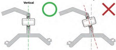
If Lift Scale is tilted and not completely vertical when installed, this will cause the joints of the Lift Scale to bend. This will eventually cause breakage once used enough times and subjected to enough weight, because force is being applied against joints in a way that they aren't designed to handle.
