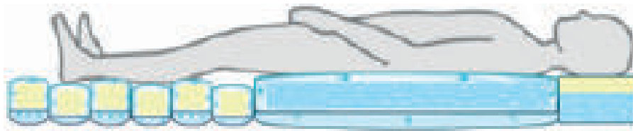
Figure 1: Diagram of three different regions of support in the FLEXI by Pure Air mattress (head, torso & heel).
