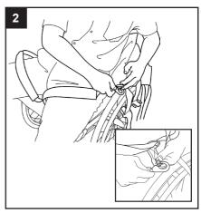
Attach the leg supports to the Standing Harness by offering the safety clasp to the retaining ring at the bottom of the Standing Harness as shown. The leg supports can be adjusted in length for comfort as appropriate.
