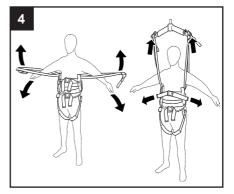
To attach the Standing Harness to the spreader bar, firstly place the patient's arms through the loop straps as shown, and attach to the spreader bar by using the coloured loop straps. Ensure the same colour loop is used on both straps and hook onto the side hooks. Check both loops are securely attached prior to use.
